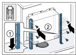
10. Screw the rails onto the bottom of the unit.
