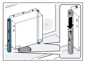
**11. Note:** If an appliance measuring 90 cm is installed in a unit with a width of 90 cm, skip the next two installation steps and follow the instructions in the additional accessory pack.
