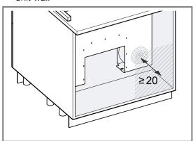
Include a ventilation opening in the base with a cross-section of 80 cm<sup>2</sup>.
