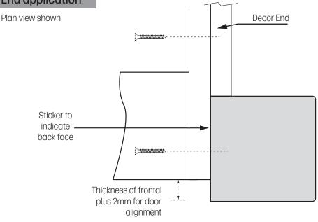
Any cut or exposed edges must be sealed to avoid moisture ingress
