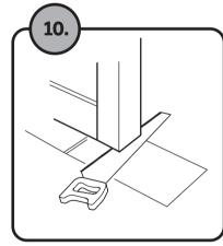
**Door frames** down) next to the door molding and saw as shown. Slide the tile under the moulding.
