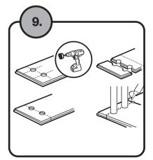
**Holes for pipes** Measure the diameter of the pipe and Lay a board (with the decorative side drill a hole that is 6mm larger. Saw the board removing the piece, lay the board, then re-fit the sawn piece.
