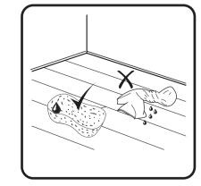
Do not use excessive water when cleaning, use cleaners recommended for laminate floorina.
