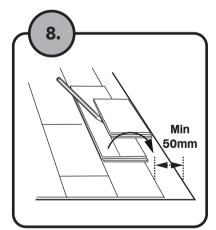
Last Row Use a board to mark the width of the board to be cut. The last row should be at least 50mm wide. The spacers can then be removed. Note: Use a pull bar to ensure last row is in place.
