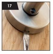
Make sure the roses on both levers are flush to the door and tighten the grub screw on the lever you just attached.
