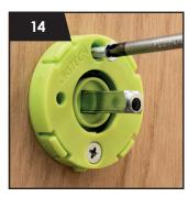
Secure the sprung cassette using the two machine screws provided. **TIP:** Do not over tighten the screws or damage to the cassette could be caused.
