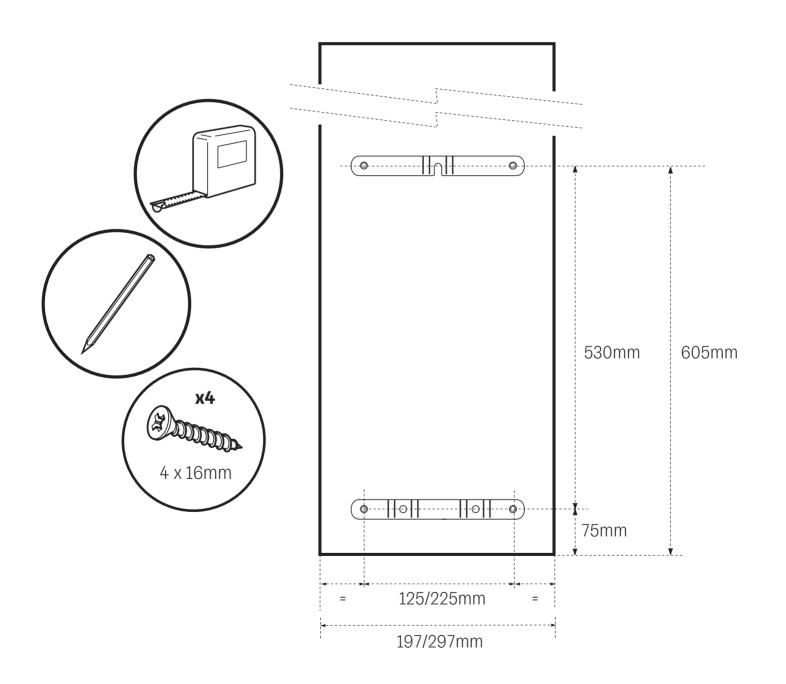
Fit the door slotting the bracket onto the frame at the top.
