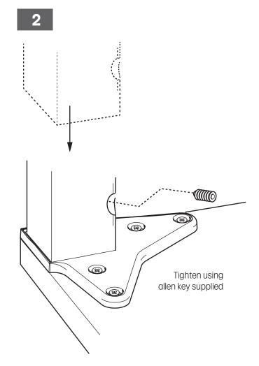
**Note:** The leg can be modified in height by removing the foot bung and cutting to the required height (from the bottom edge). Once cut, re-fit the foot bung.
