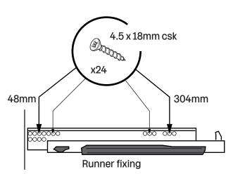
Fit brackets to the underside of drawer.
