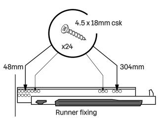
Fit brackets to the underside of drawer.
