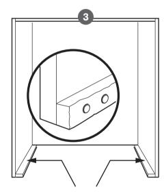
Carefully remove final sections of base panel and trim back dowels.
