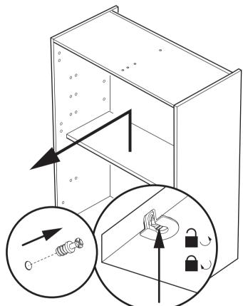
Drill through fixing holes in the top of the cabinet.
