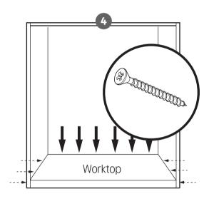
Measure, cut and fit required worktop panel, securing with screws or adhesive each side and back.
