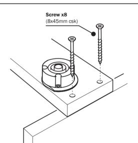
Mark and fit brackets to the back of drawer front. Secure the front to the drawer box then fit the drawer to the runners.
