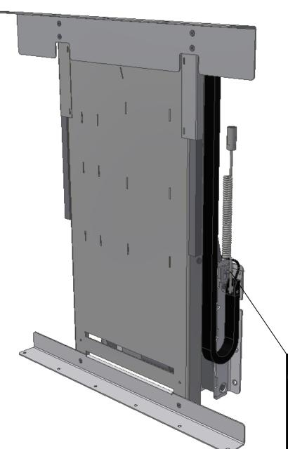
Loosen the nut that keeps the cable track in place, pull cable track aside
