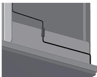
Connect extension cable of control box to safety stop plate on the left side (shown from the front) and fasten it with cable binders as shown on page 21
