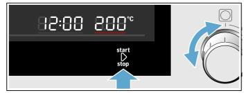
The appliance will start heating. The start  $\triangleright$  stop LED will be lit. The length of the bar on the temperature indicator gradually increases.
