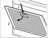
3. Slightly tilt the front of the filter downwards (2), then pull.
