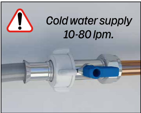
Ensure water is turned on and the isolator valve is accessible after fitting. Hose connection - 3/4". Cold water pressure - 0.3 -10 bar (0.03-1.0 Mpa)
