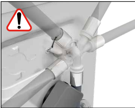
NOTE: If necessary loosen and rotate the water hose towards the water supply and re-tighten. (Always use the new hose supplied with the washing machine).
