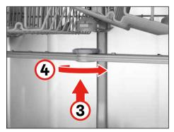
**Lower spray arm** (\*Only rotate by gripping centre of spray arm)
