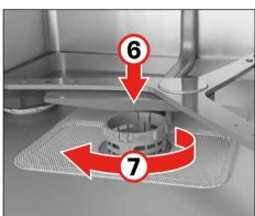
Caution: The dishwasher must not be used without filters. Incorrect repositioning of the filters will produce poor washing results.
