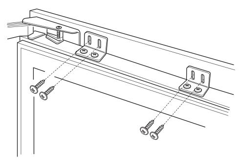
Due to the lower door brackets clashing with the edge of the kitchen door panel, we recommend the larder brackets are used to secure the door at the top and bottom. **Note:** Ensure spacing of door (top and bottom) is equal.
