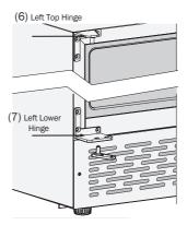
Turn the glass door 180° and reinstall using the pivot plate, tighten screws to secure the hinge plate.
