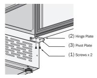
Pull down to remove the glass door and place it on a padded surface to prevent scratching it.
