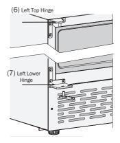
Turn the glass door 180° and reinstall using the pivot plate, tighten screws to secure the hinge plate.
