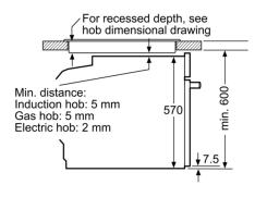
measurements in mm
