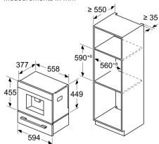
Measurements in mm Left corner installation ≥ 350 100 110°
