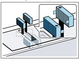
6. Insert the grease filter.
