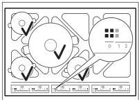
For the combination indicated above, there are four active control bars. The left front pot is indicated by A indicator visible on the first control bar. The left rear pot is indicated by B indicator on the second control bar. The middle pot is indicated by indicators A B C D visible on the third control bar. The right front pot is indicated by C indicator visible on the fourth bar.
