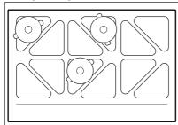
Medium-sized cookware with the bottom diameter between 160 mm and 210 mm should be placed on a pair of triangles.
