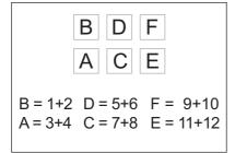
Zone indicators indicate which standard cooking zone is controlled by the appropriate control bar. The hob has 6 control bars.
