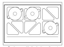
Cookware with the bottom diameter between 240 mm and 350 mm should be placed on four triangles.
