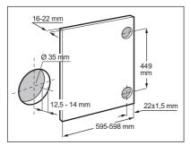
Set the position of the lower hole respecting dimensions and distances shown in the drawing (449 mm).
