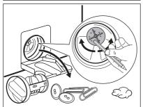
**7.** If it is necessary, remove fluff and objects from the filter recess.
