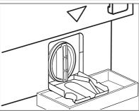
2. Place a suitable bowl below the drain pump access to collect the water that flows out. Always keep a rag nearby to dry up any water spillages when removing the filter.
