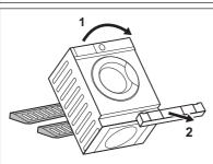
**3.** Remove the polystyrene protection from the bottom.
