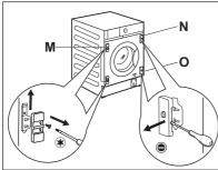
If the cupboard door has to be opened from left to right, invert the position of the hinge supports M with the magnetic plate N and lower plate O.
