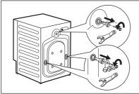
**6.** Remove the three bolts, the hose holders and plastic spacers by using the spanner supplied with the appliance.
