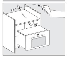
Slide the microwave oven into the niche. Feed the cable with the plug through the back of the unit.
