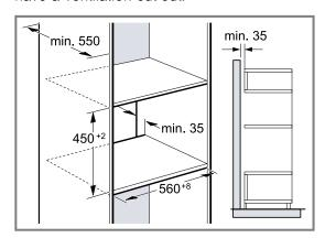
If the tall unit has another back panel in addition to the element back panels, this must be removed. Do not fit the appliance too high up; it must be possible for accessories to be removed easily.
