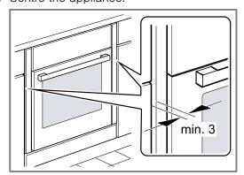
There must be an air gap of at least 3 mm between the appliance and adjacent cabinets. 3. Screw the appliance into place.
