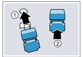
**3.** Hook the rear retainers with the hook into the top hole ① and push them into the bottom hole ②.
