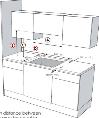
Minimum distance between cabinets must be equal to overall width of all hobs.
