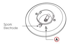
In case of flame failures of the burners for any reason, the flame failure sensor (A) will cut off the aas flow after a few seconds.
