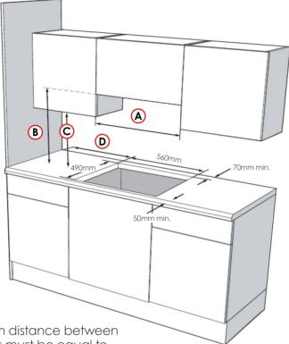
Minimum distance between cabinets must be equal to overall width of all hobs.
