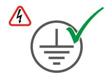
**WARNING!** This hob must be connected to an earthed mains supply in accordance with the product technical specifications.
