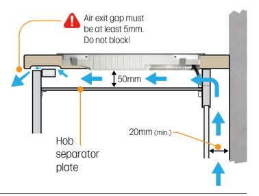
**Ventilation is very important:** We recommend (in addition to the instructions shown in the Kitchen Installation Manual), that further ventilation is made possible by modifying the cabinet as shown.
