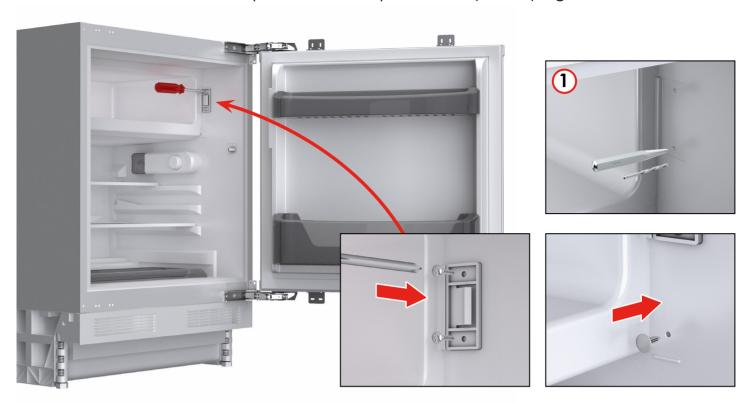
4 - Carefully, using a centre punch or pilot drill the pre-marked hole on the side wall, 1.
