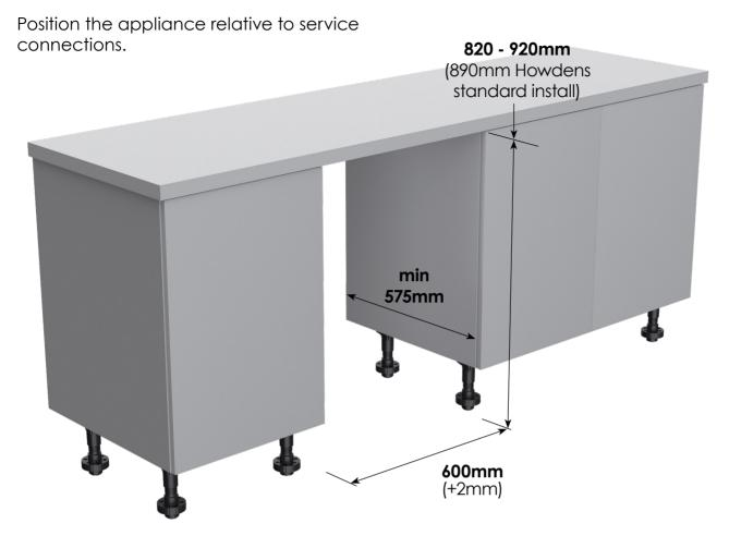
**Note:** If opening against a wall, **180mm** clearance is required to allow the baskets to be removed.
