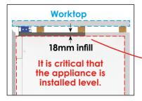
**Note:** For profile kitchens - insert 18mm board below worktop, level with bottom edge of front panel.
