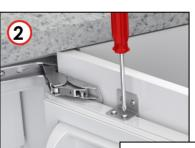
Loosen top bracket screws and slide left/right to achieve frontal alignment. Secure when positioned correctly.
