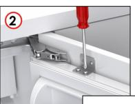
Loosen top bracket screws and slide left/right to achieve frontal alignment. Secure when positioned correctly.
