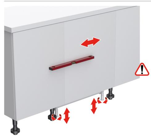
If necessary, make minor adjustment so the door frontal is aligned with the door frontals alongside.
