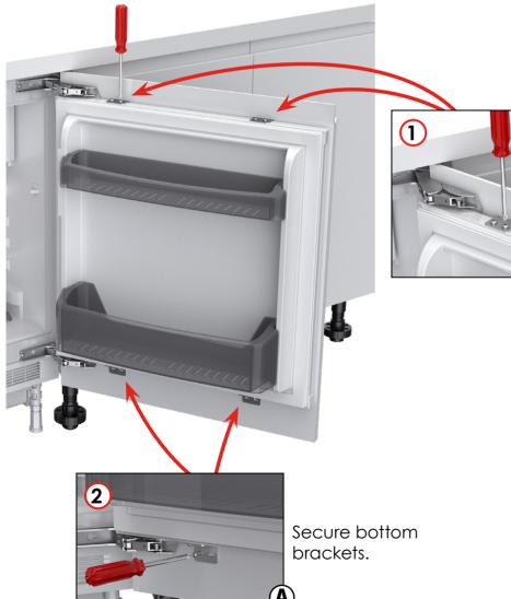
Attach frontal to the appliance door and slide left/right to achieve frontal alignment. Secure when positioned correctly.
