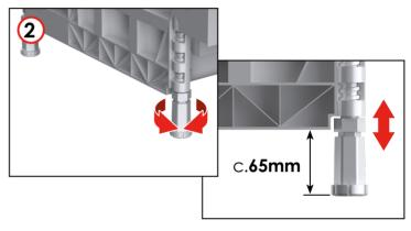
IMPORTANT: Do not use extension feet for Profile Kitchens and when fitting a granite/solid surface worktop, see stages 5d/5e.
