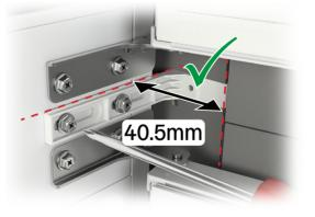
Please use brackets with tabs to ensure fridge freezer install depth is 40.5mm. (Use front feet adjustment to assist)
