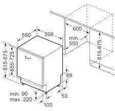
measurements in mm
