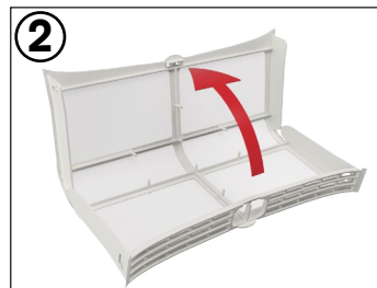
2 Open the filter. Gently remove any lint using a soft brush, vacuum or use your fingertips.
