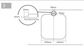
Using the dimensions shown, cut out the rebate for the overflow pipe from the underside of the worktop.
