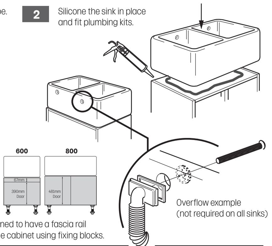
**Note:** The 600 belfast sink base cabinet is designed to have a fascia rail fitted above the door. This fascia is secured to the cabinet using fixing blocks.
