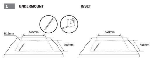
**Note:** Measure cut dimensions against the sink to ensure correct. Undermount sink dimensions can change, depending on the overhang preference.
