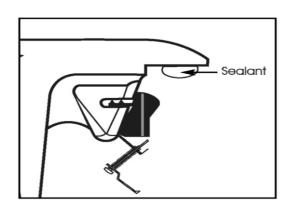
5. Apply a bead of "Silicone sealant" (not included) to the underside of the sink flange. For final fit, make sure each sink clip is pulled back as illustrated. Position the sink into the work top opening.
