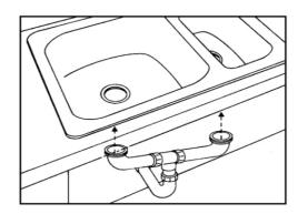
7. Make water and waste pipe connections as required.
