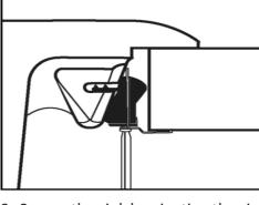
6. Secure the sink by pivoting the sink clips into the position illustrated and tighten screws in the front, then tighten rear and side screws.
