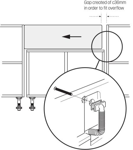
Re-align sink to the cabinet and connect waste plumbing kit and overflow. 7 Fit the decor end panels each side of the sink base cabinet and secure to base cabinets from the inside, using 30mm screws.
