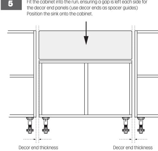
Fit the cabinet into the run, ensuring a gap is left each side for
