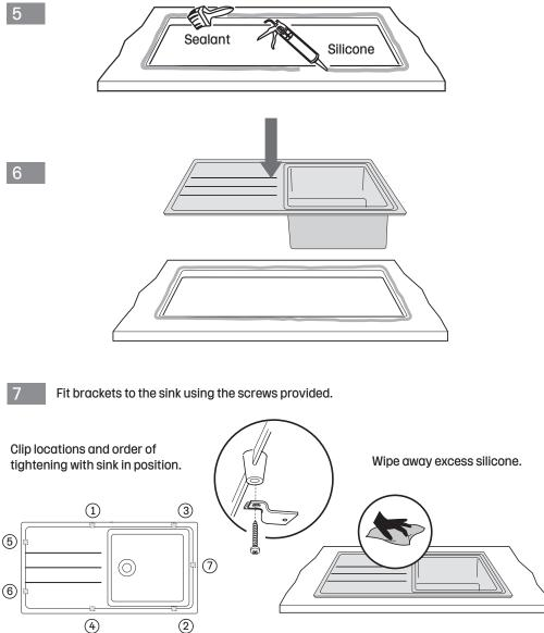
Note: Once tightened, brackets can be secured up into the underside of the worktop. Screws are not supplied.
