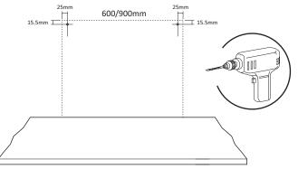
Using the dimensions shown, mark the fixing positions and drill holes suitable for appropriate wall plugs.
