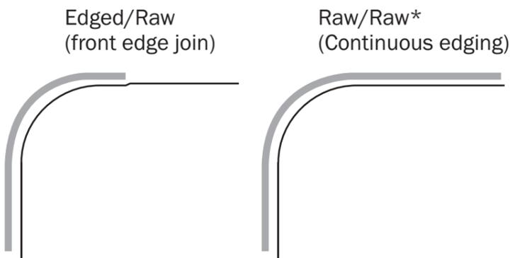
\*Working with a raw front edge can only be achieved by using the back of the worktop as the front edge. Before using this, the backing paper will need to be removed to enable the edging strip to fix correctly.
