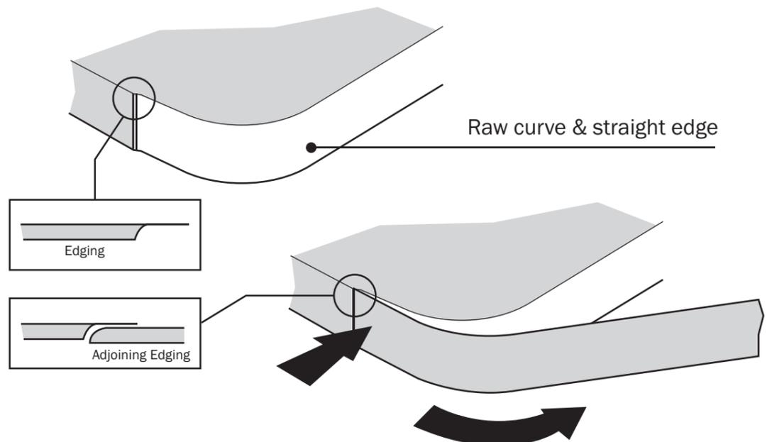
**Hints & Tips:** Once edging adhesive has been applied, warm the edge before applying the edge banding. Edging clamps can be used to ensure a secure fix.
