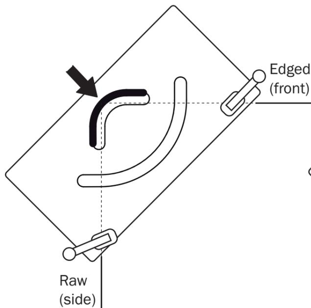
Router a smooth finish inner curve pushing the jig to the front edge (Illustrated by thick black line)
