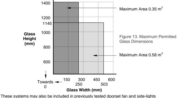
Pyrostem glass in timber based doorsets for periods of 60 minutes integrity
