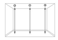
Measure your ceiling height at three points along the length of the ceiling.
