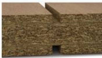
Machined grooves from each face for timber infill
