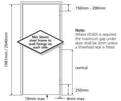
Measure from the top of the floor covering to the underside of the door.
