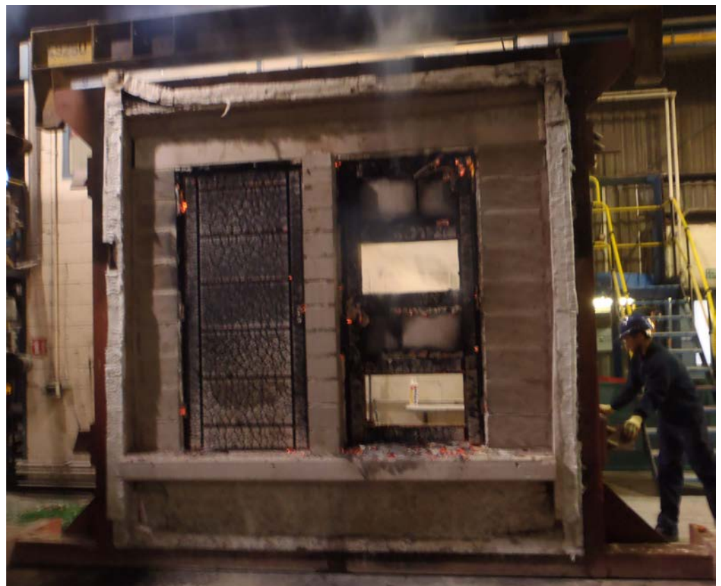
The exposed face of the doorsets immediately after the test
