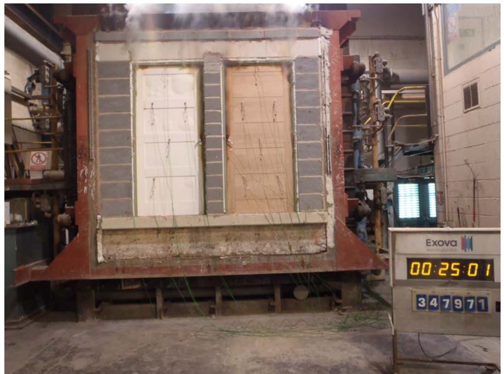
The unexposed face of the doorsets after 25 minutes of testing
