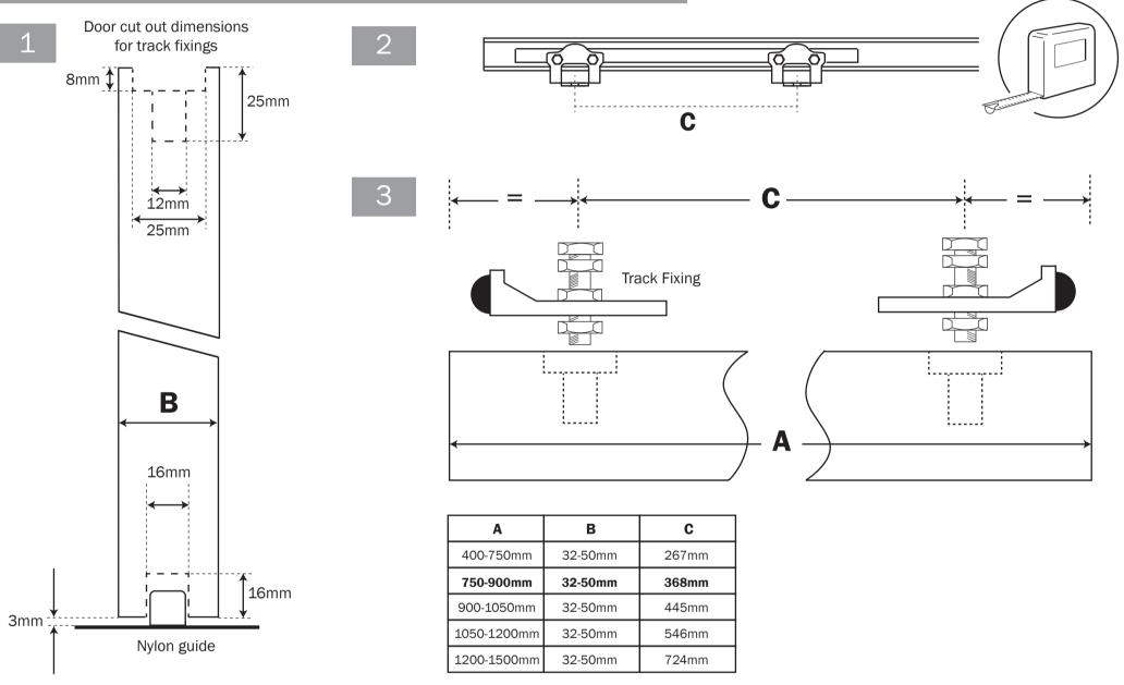
1. Using the dimensions shown in the diagram above, router the top and bottom of the door for the track fittings.
