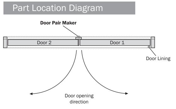
The gap between the doors should be a continuous 12mm in order for the door pair maker to be fitted.
