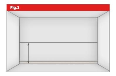
Cut dado rail to length. Apply adhesive to back of moulding and offer up to horizontal line. Secure using a nail gun (Fig 2).
