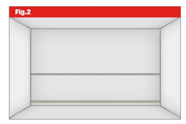
Decide how many panels you would like to run across the wall. Please bear in mind that the panels will need spacing equally. For this example we are using a spacing gap of 150mm for both horizontal and vertical spacing.
